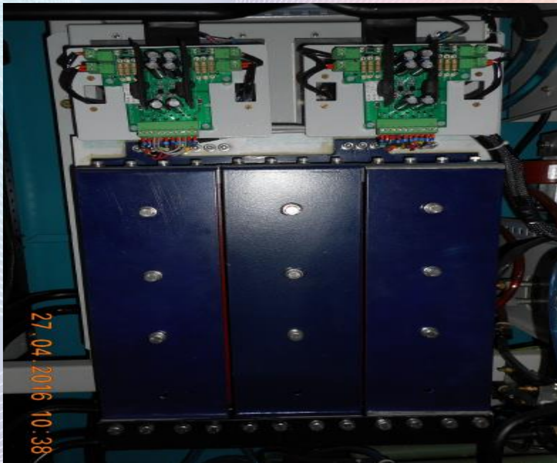
IGBT ASSEMBLY WITH DRIVER CARDS
